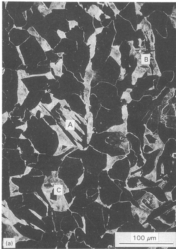
Figure 4 Scanning electron micrographs images. Note the contrast reversal with respect to Figs 1–3. (a) Low-magnification image. Three nodules (A–C) contain intragranular Widmanstätten ferrite. (b) High-magnification image of nodule A. The cementite is seen to be predominantly lamellar.
